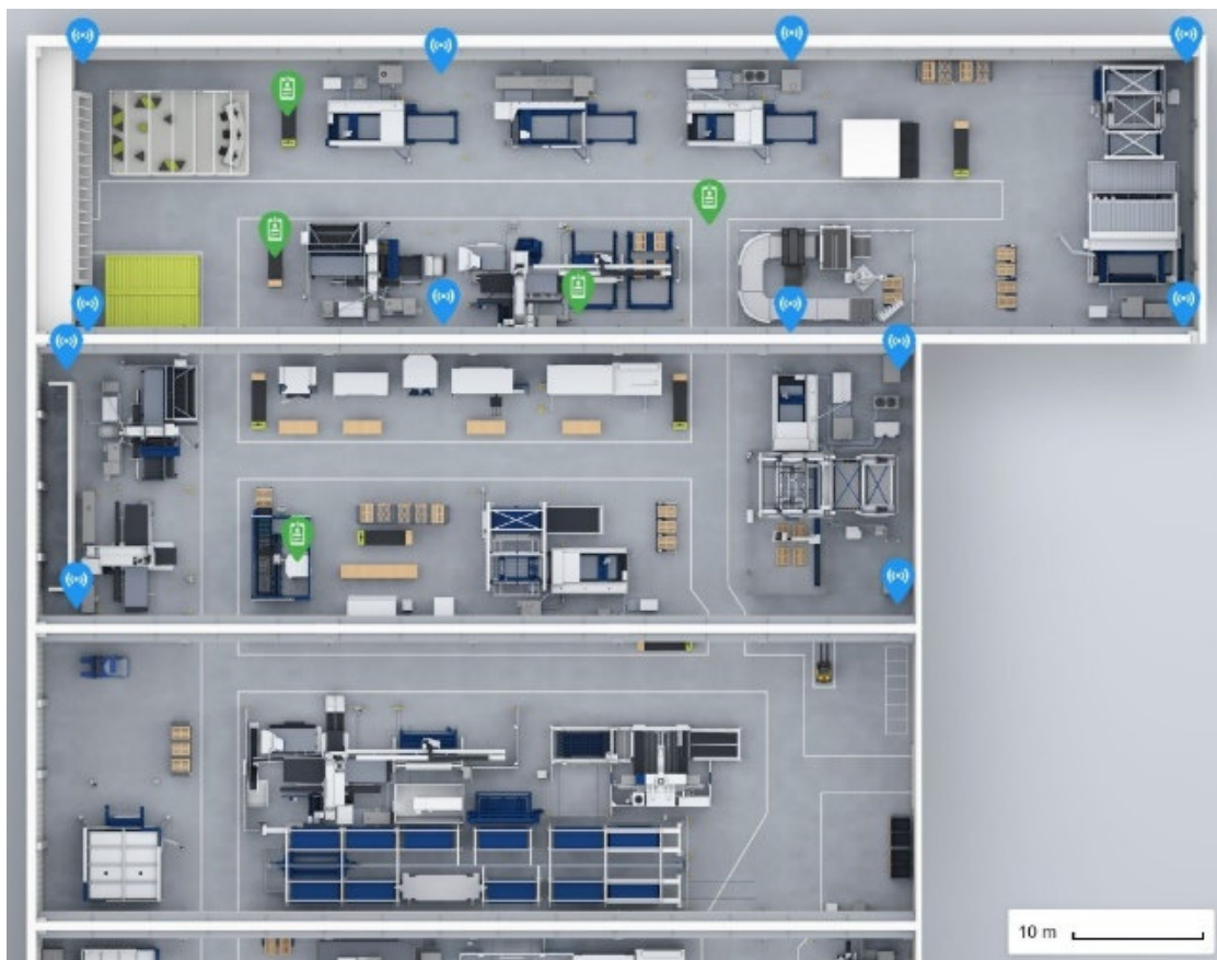
Figure 1: Exemplary integration of an omlox infrastructure (blue flags) with localized omlox tags (green flags) on the shopfloor
