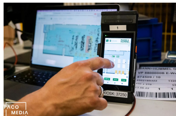
Figure 10: The scanners used at MANN+HUMMEL (equipped with an omlox tag) to locate stored goods
